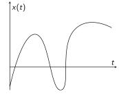
In analog systems, information is contained in a continuous waveform...
